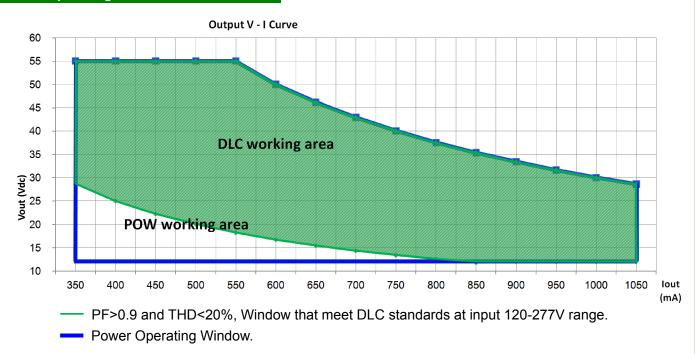
Note: When the output current is set, the output voltage is automatically limited within the curves.
