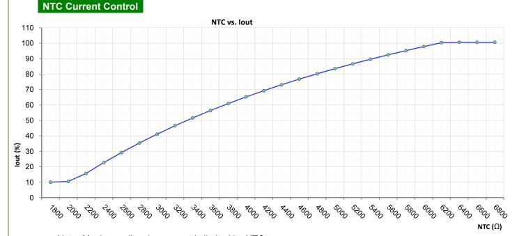
Note: Maximum dimming current is limited by NTC. NTC values, NTC High, NTC Low and NTC Minimum lout can be programmed. Using YG Programmer USB interface & YG PC based GUI Software.
